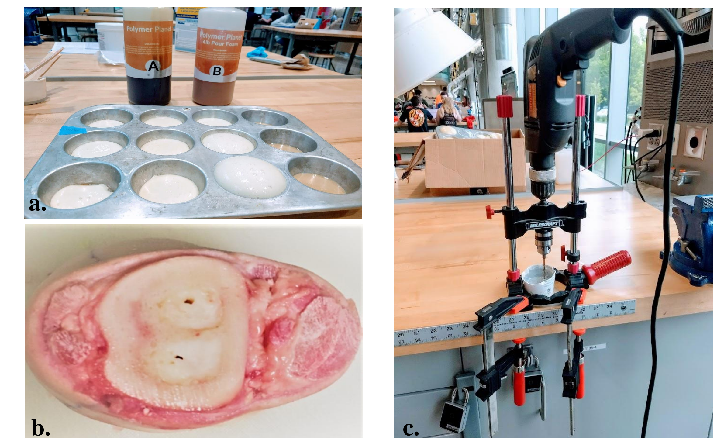
Figure 7. (a) Polyurethane foam ratio testing for inner bone composition of osteoporotic patients. (b) Cow bone used for inner and outer bone comparison testing. (c) Drill test conducted on epoxy resin coating for outer bone composition of osteoporotic patients.
