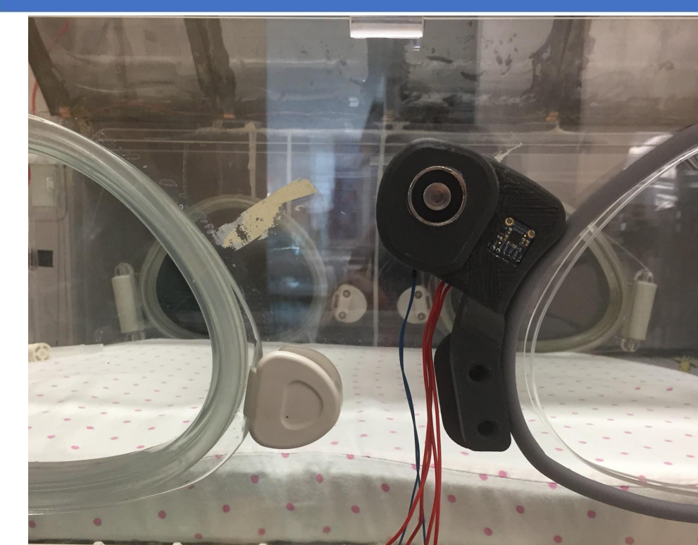
Figure 5. Prototype design mounted on isolette next to original latch.
