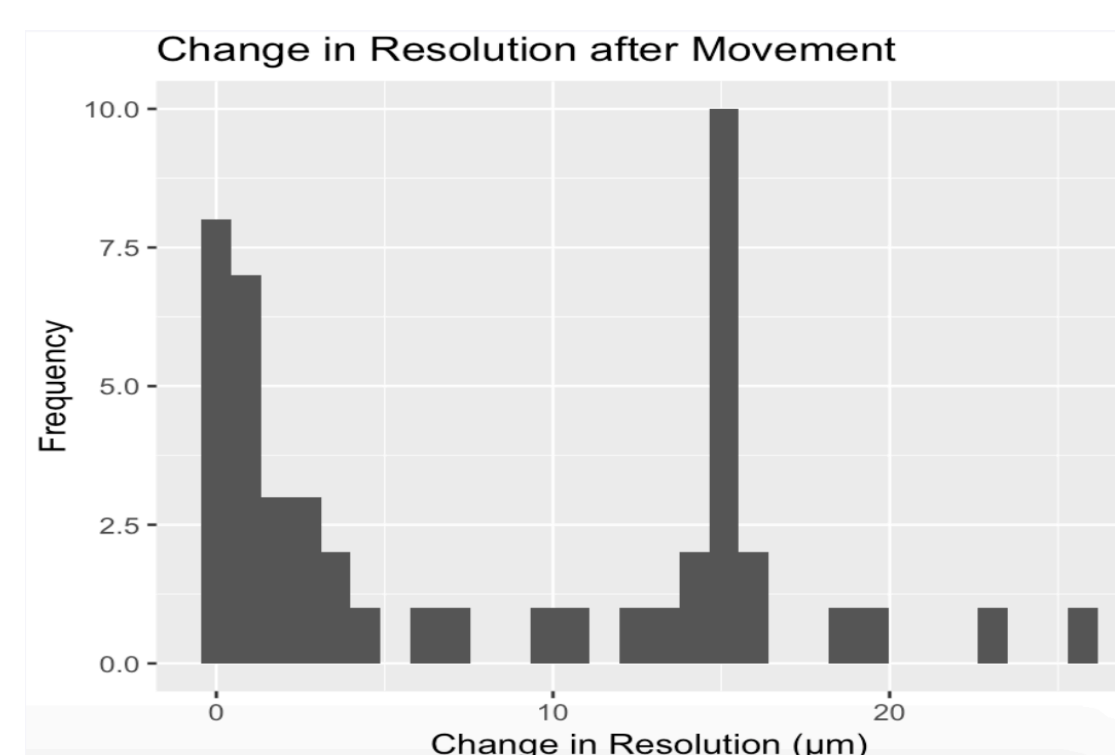
Figure 7. Histogram of change in size of smallest resolvable element after resetting lens holder.
