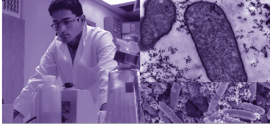
LEFT: ROHAN FERNANDES. TOP RIGHT: TRANSMISSION ELECTRON MICROSCOPE IMAGE OF THE MAGNETIC NANOFATORIES (SMALL, DARK CLUSTERS) ATTACHED TO TARGETED E. COLI CELLS. TOP LEFT: SCANNING ELECTRON MICROSCOPE IMAGE OF THE NANOFATORIES (WHITE CLUSTERS) ATTACHED TO THE SAME CELLS.
